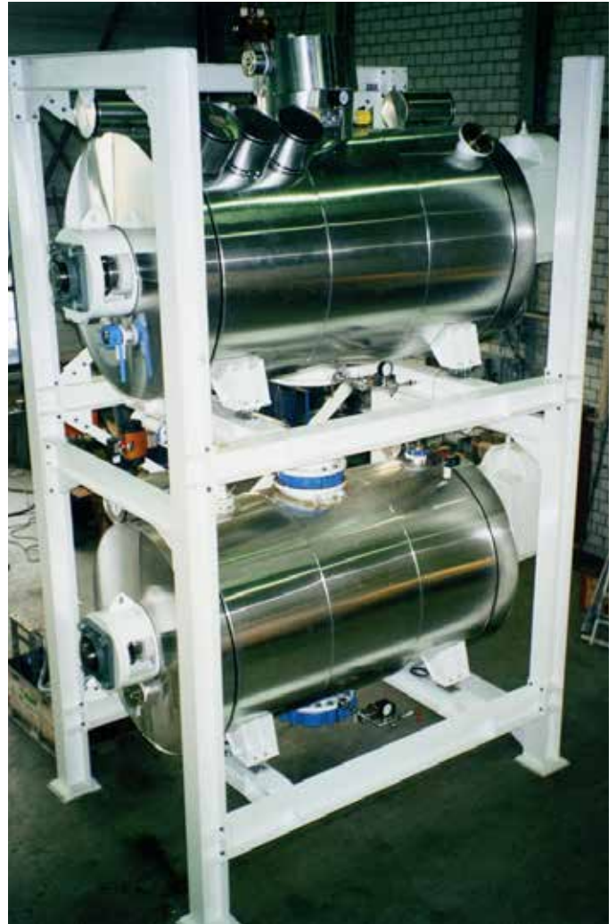
Tower construction with the Vacuum Mixing Dryer VT (above), and the Vacuum Mixing Cooler VK (below)
